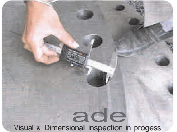
Visual & Dimensional inspection in progress
